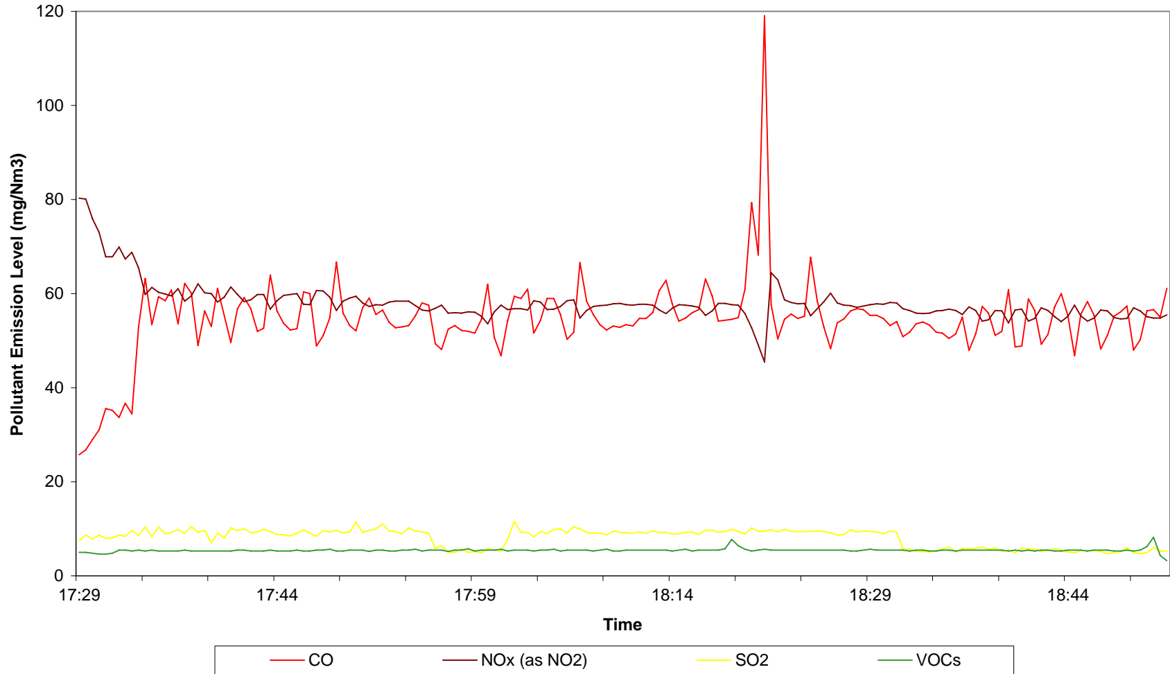
Figure 2 Combustion Gas and VOC Emissions from Rotoman 2, Upper Wyndeham Heron, Maldon (01/09/2009)
